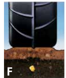
F Verify press wheel (if equipped) function ( F ).
