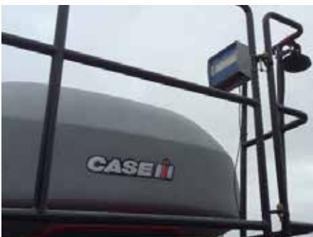
Tank fill level measurement for higher productivity with bulk seed
