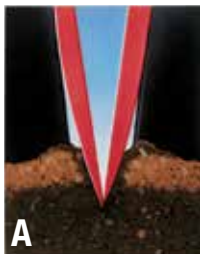
A Check depth on seed trench opening disks ( A & B ). Seed depth should be checked from the press wheel impression to the seed. Do not measure from the gauge wheel impressions, or the surface of the soil between the row unit gauge wheel tracks.
