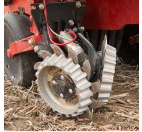
Floating No-Till Residue Managers with Depth Band (with or without air cylinder)
