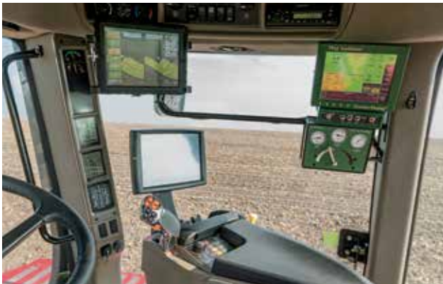
Shown are the AFS Pro 700, 20/20 SeedSense, and iPad with FieldView cab app
