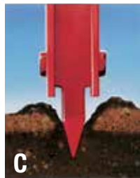
C Check furrow forming point depth ( C ).
