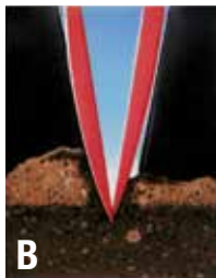
A Check depth on seed trench opening disks ( A & B ). Seed depth should be checked from the press wheel impression to the seed. Do not measure from the gauge wheel impressions, or the surface of the soil between the row unit gauge wheel tracks.
