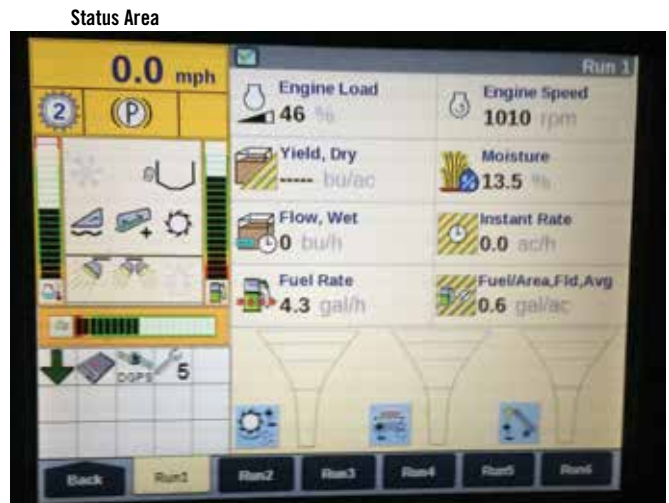
Alarm Status Area
