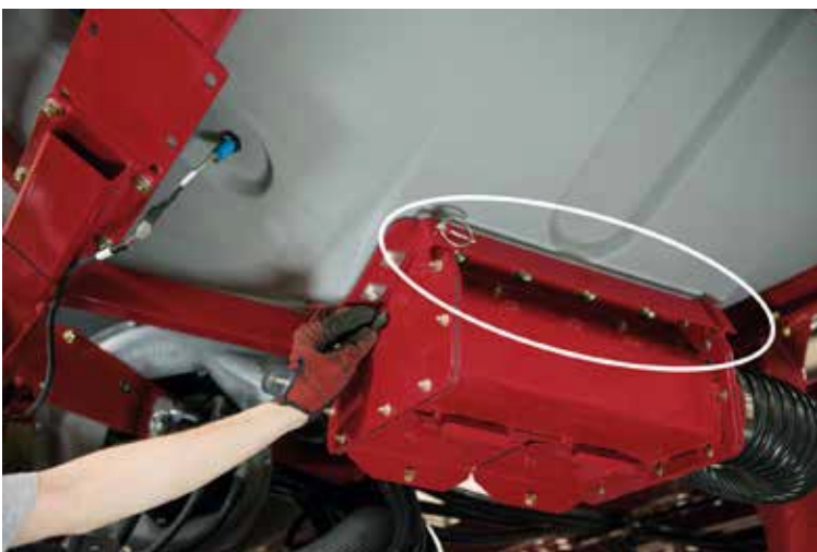
Blockoff Plate Stored
