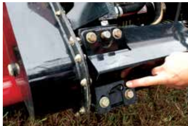
Change Gearbox oil level every 600 hours or every year
