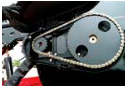
Lube reel chain drive every 10 hours
