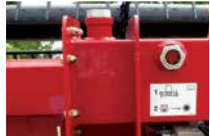
Check reservoir through the sight glass every 10 hours (step 2)
