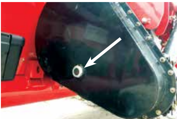
Change auger drive chain case every 600 hours or every year
